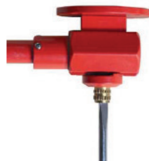
Loosening the inner screw so that the "Mexican" can be turned.
